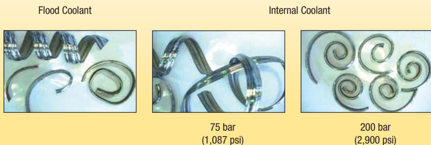
Material steel ST52; Insert size 6mm; f = 0,25 mm/U
