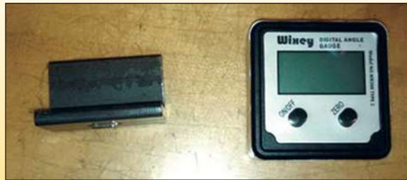
Figure 1: Angle finder seat (left) and digital angle finder (right)
