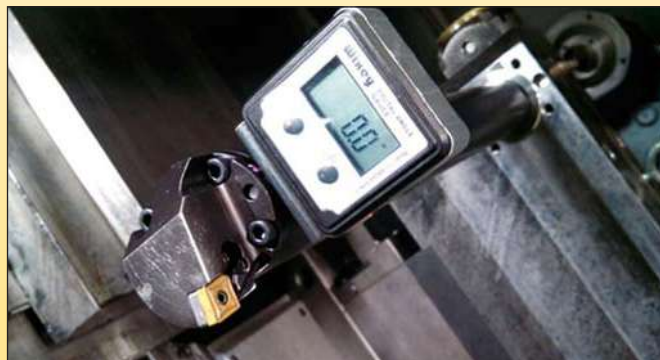
Figure 4: Aligning the boring bar
