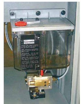
MQL Microlubrication system. Available for all series.
