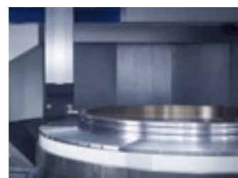
RAM_ Made in forged steel to optimize the balance between rigidity, damping capacity and dynamic behavior. Sections available: 320 x 320 / 400 x 400 mm. Travels up to 1500 mm.
