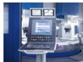
Fix and rotating control panel in the left side for an optimum interaction with the operator. 19" touch screen.
