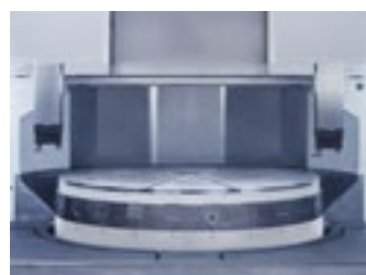
Cast iron made turning plate with radial T-slots (clamping fixtures not included in the standard configuration).
