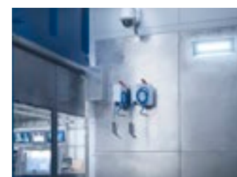
• Surveillance cameras within the working area controlled from the dashboard console. • Full stainless steel lined working area, including protection bellows.
