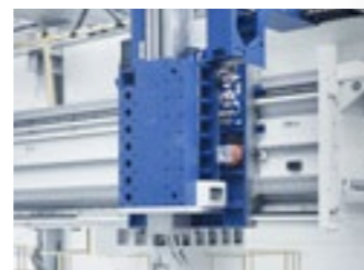
Cross-beam_ The high rigidity fixed cross-beam is made of casting GG-30 for hydrodynamic guiding system or in steel-welded for hydrostatic guiding system as option.
