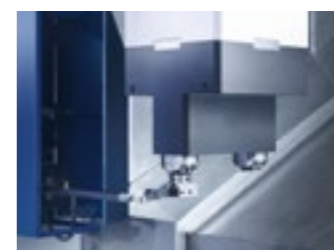
Different tool measuring, spindle control and piece inspection systems integrated in the machine.
