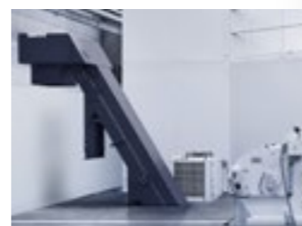
Chip Conveyor with integrated coolant tank. The chip extraction is realized by paddle turning around the rotary table.
