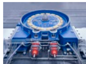
Main spindle_ The guiding of the upper plate during the rotation is realized by a radial load bearing and hydrostatic system.
