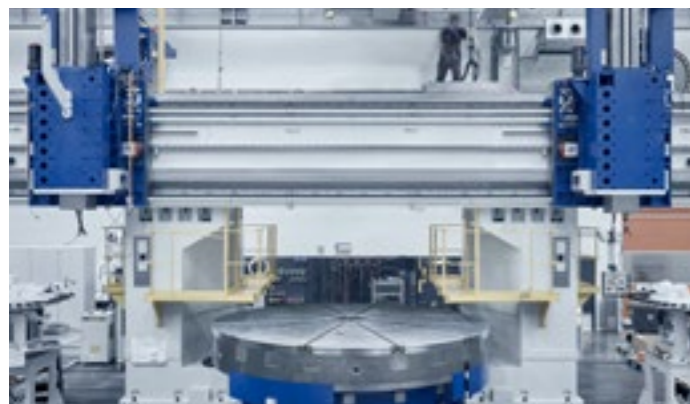
Main spindle_ The guiding of the upper plate during the rotation is realized by a radial load bearing and hydrostatic system.
