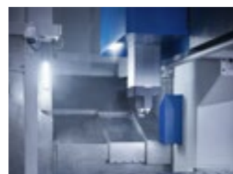
• Working area lightning with lamps inside the working area and led under crossbeam. • Watter and air guns.
