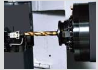
Auto tool damage detection device II (OMRON) option
