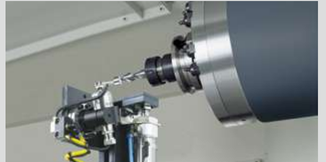
Automatic tool measuring device (TS 27R) option
