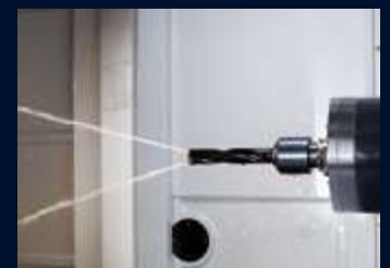
Spindle-through coolant spray device option
