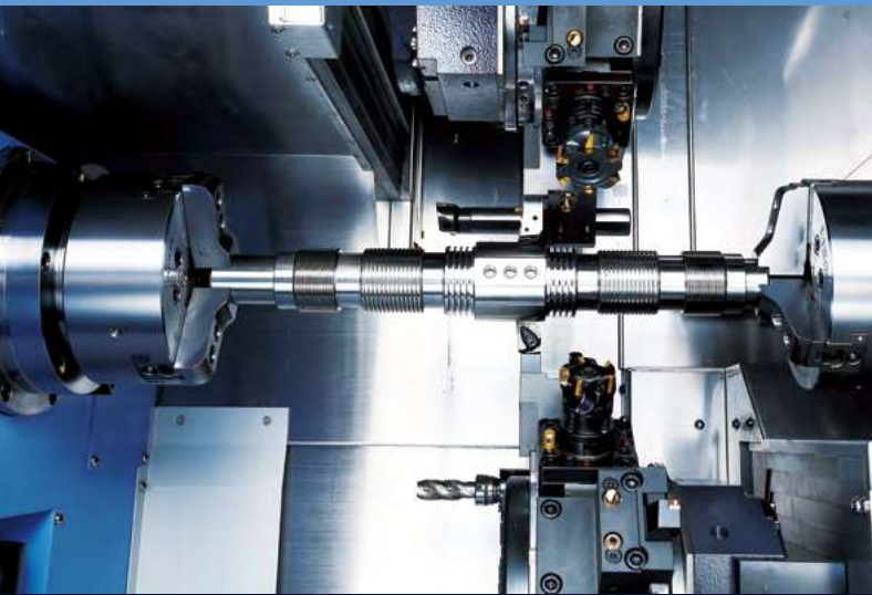
Turning at the same position is carried out using the upper and lower turrets simultaneously.
