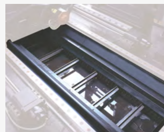
Internal Chip conveyor OPTION (SCRAPER/HINGED)
