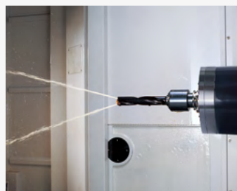
SPINDLE-THROUGH COOLANT (TSC) OPTION
