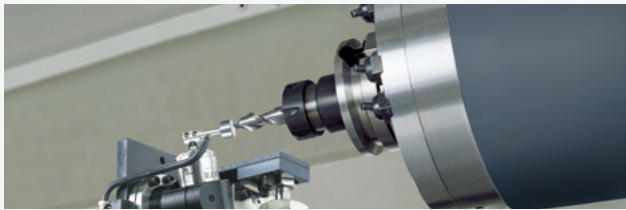
AUTOMATIC TOOL MEASURING DEVICE (TS 27R) OPTION
