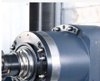
COOLANT FLUSHING ON THE SPINDLE HEAD
