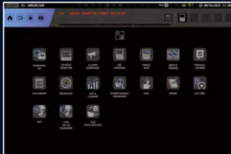
**Supports various apps in three fields—setup, machining and utility**
