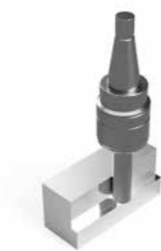
Material: Aluminum alloy Tool: ø16 end mill Conditions: S3950 min -1 F1550 mm/min
