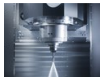
Coolant through spindle (22 bar).
