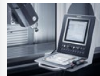
Heidenhain TNC 640 HSCI control.
