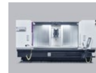
Vertical headstock 3 axis option for basic machining operations at an affordable price (STAR 3000).
