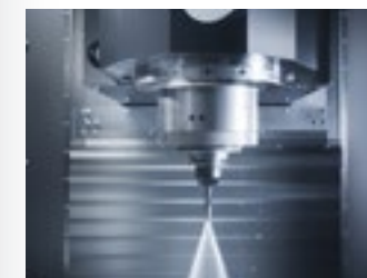
Coolant through spindle (40 bar).
