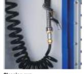
Cleaning gun Helps clean the workpiece or chips inside the machine after machining.
