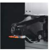
Head coolant nozzle with head shower Coolant can reliably be applied to the machining section as the tool and nozzles are set in place. In addition, a head shower is provided to remove chips from the head.
