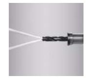
Coolant Through Spindle (CTS) Can be selected from 3 MPa or 7 MPa. Pump and tank are not included. \* 7 MPa CTS option is available only for the BBT spec.
