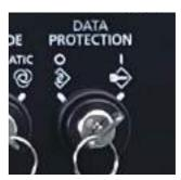
Data protection switch, key type Changing the operation level is enabled or disabled by the key.
