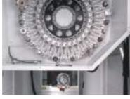
Equipped with the newly developed direct ATC type 30-tool magazine. Supports maximum tool length of 250 mm, maximum tool diameter of 125 mm, and maximum tool weight of 4 kg, enabling a variety of machining, including long workpieces.
