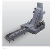
Chip conveyor A two-step structure (hinged plate and scrapper) is used, enabling evacuation of chips in a variety of sizes and shapes. An oil skimmer can be added.
