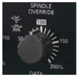
Spindle override Spindle speed can be changed without changing the program.
