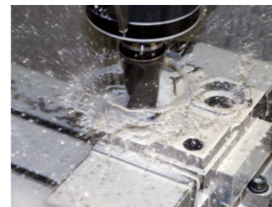
Large hole drilling using high-torque specs
