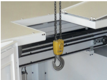
Top loading door for crane operation.
