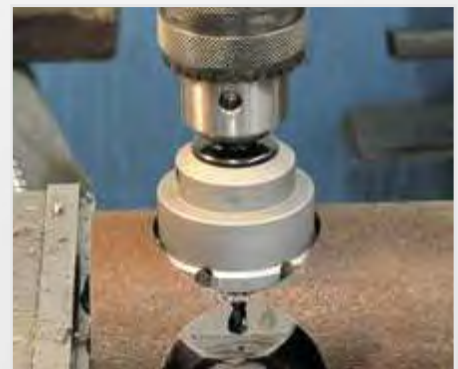
Drilling in pipes
