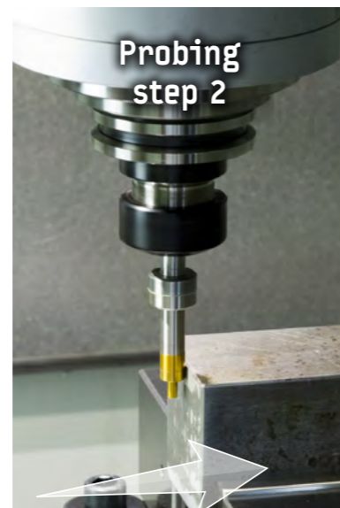
2. By slowly and carefully approaching the rotating edge finder to the respective reference surface, the oscillation movement steadies successively.
