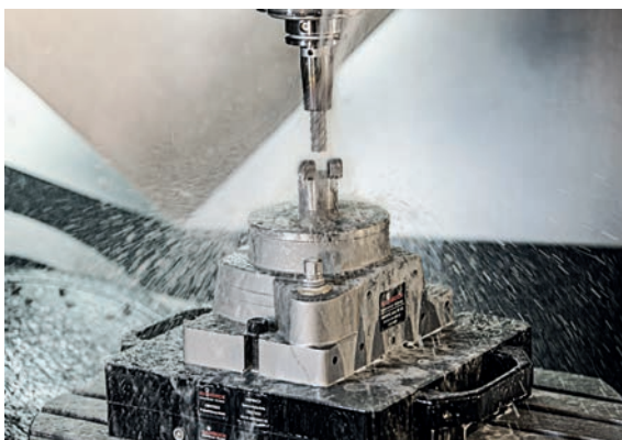
MANOK plus manual stationary chuck in use
