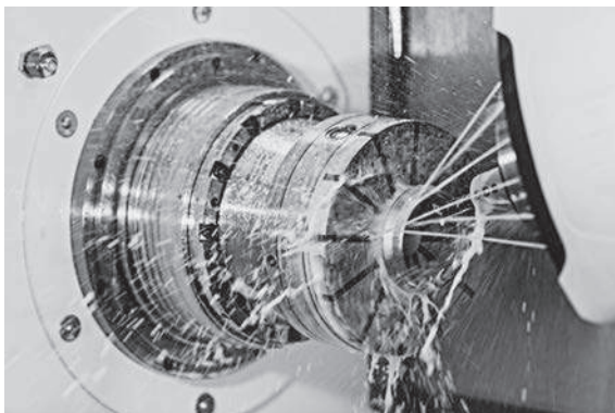
Magnet module in use
