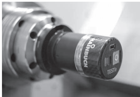
Mandrel MANDO and TESTit in use
