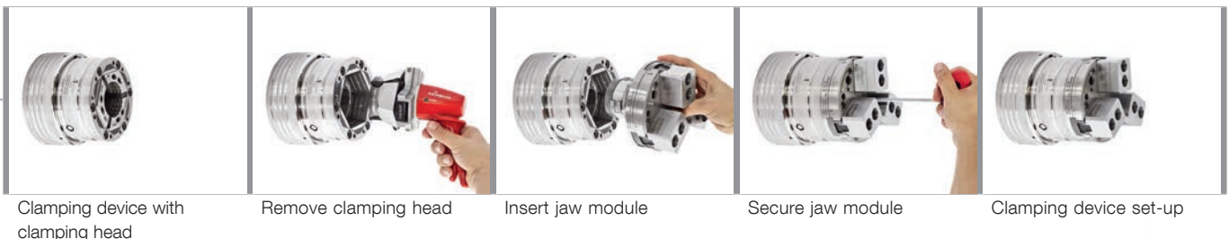
Fit on segmented clamping bushing
