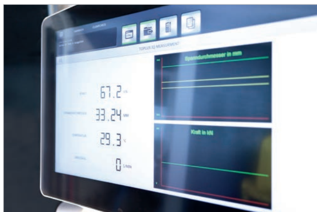
Condition monitoring on the machine controller
