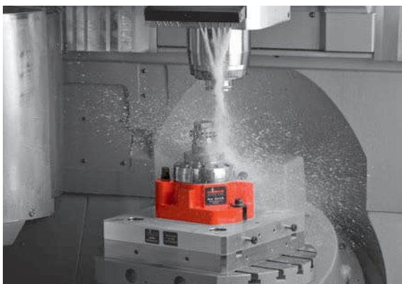
ms dock mandrel actuating unit in use
