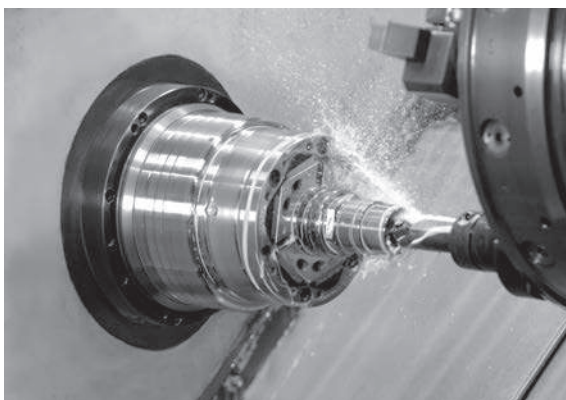
TOPlus combi pull-back chuck in use
