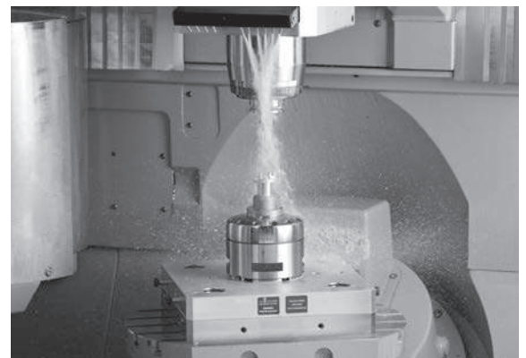
hs dock mandrel actuating unit in use
