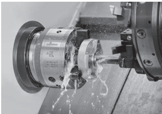
B-Top jaw chuck in use
